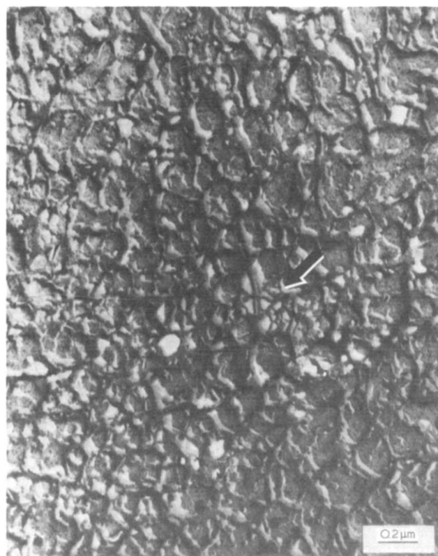
Figure 1 Electron micrograph from a polyacrylamide gel composed of 5% polymer in water with a crosslink to monomer ratio of 2.66%. (Magnification 58\,000\times )
